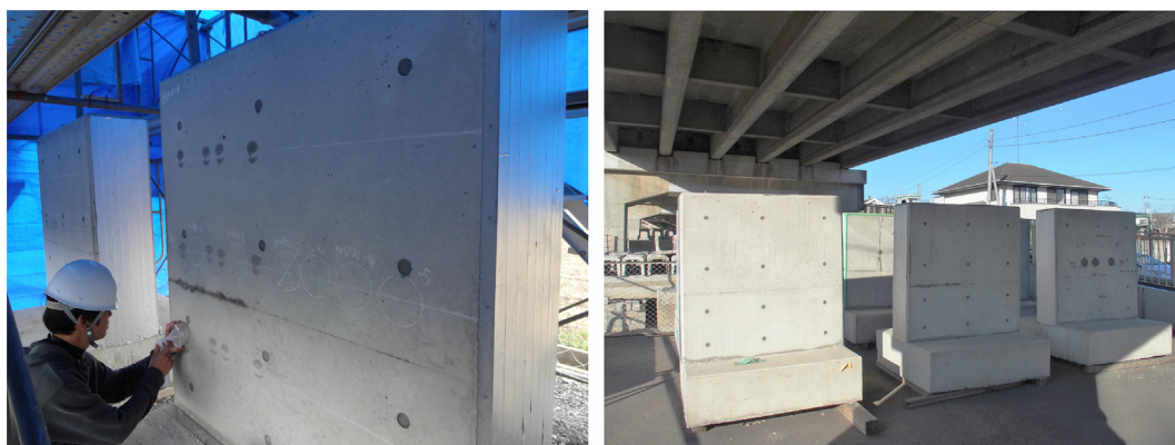
Fig. 2. Outline of specimens: under a tarpaulin until the age of eight months (left) and under a bridge girder thereafter (right).
